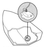
Inside the Hull Mounted Transducer
